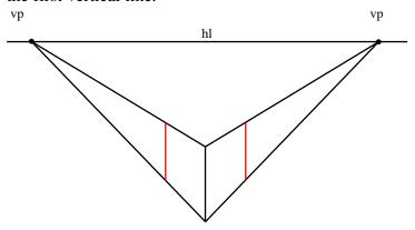
6) Draw two more lines, one from each VP to the top of the new VL on the far side of the central vertical line.
