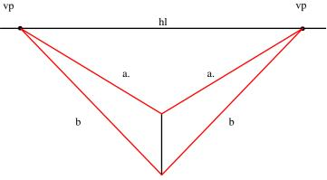
4) b. Draw a straight line from the bottom of the VL to each VP.
